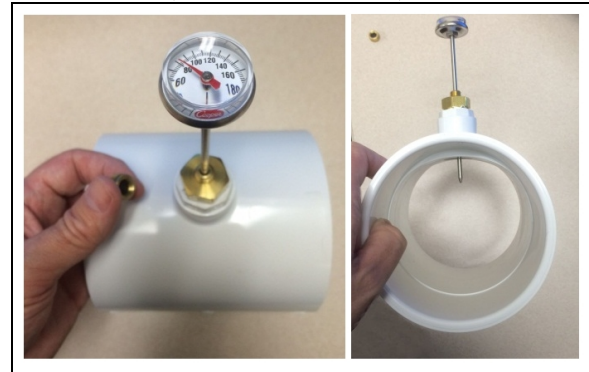
Temperature Port (Shown with Probe)
