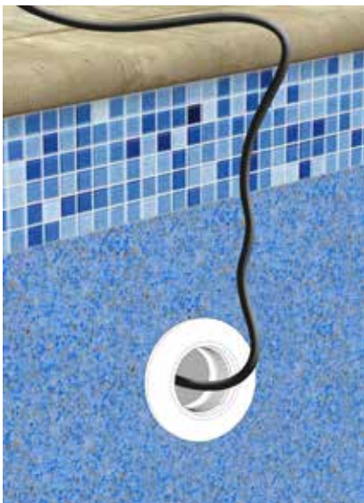
Diag 1. Existing 1 1/2" female thread in pool wall, cable extended to deck.
