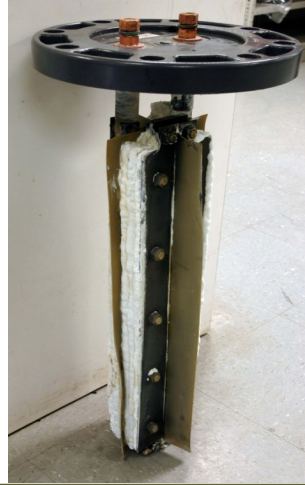
A cell stack with calcium bridged plates that requires cleaning.
