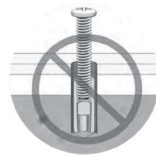
FIGURE 2 IF SCREW HOLE HAS DAMAGED THREADS
