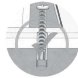
FIGURE 4 ENSURE AT LEAST THREE THREADS OF ENGAGEMENT AND HAND CHECK TO ENSURE SCREW IS SECURE
