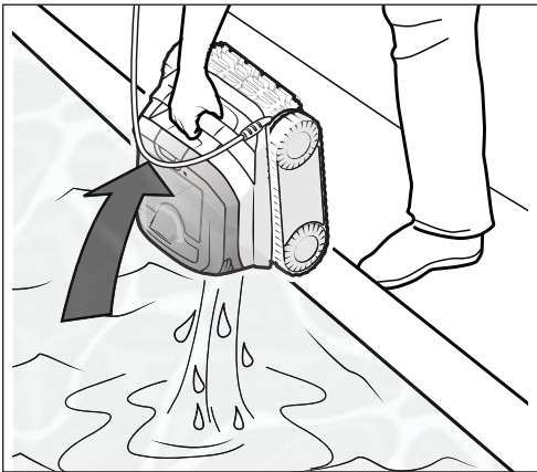
Figure 6. Always Remove Cleaner Using the Handle
