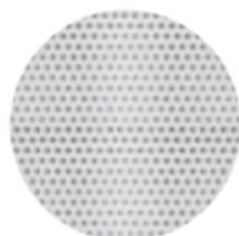
180µm Nylon filter high permeability, traps large dirt
