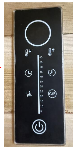
Sauna Control Panel has no Illumination
