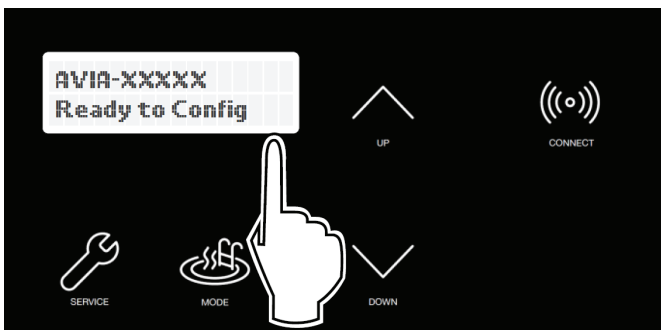
Figure 80. Wi-Fi Ready to Configure and HOTSPOT Identifier
