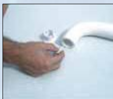
6. Apply adhesive to inside surface of safety/exercise bar.
