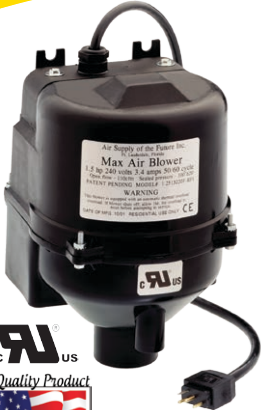
Air enters through the bottom of the Max Air blower creating a tortuous path, trapping noise inside the blower
